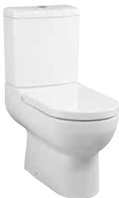
Ancona Washdown Rough-in: Fixed Bottom 190/250mm, Horizontal 180mm WBSEAC11.WW ✓✓✓
