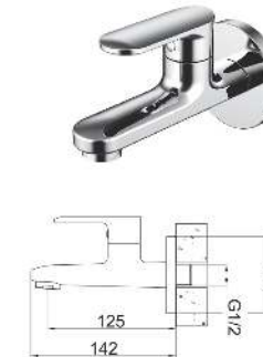
175.05101 CP brass wall mounted bib tap with quarter turn single lever handle and wall flange.
