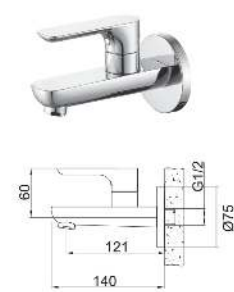
191.07101 CP brass wall mounted bib tap with quarter turn single lever handle and wall flange.
