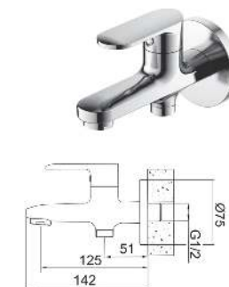
175.02101 CP brass wall mounted two way tap with quarter turn single lever handle and wall flange.
