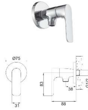
191.09101 CP brass 1/2" angle valve with quarter turn single lever handle and wall flange.
