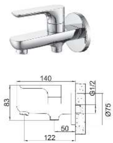
191.06101 CP brass wall mounted two way tap with quarter turn single lever handle and wall flange.
