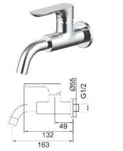
191.05101 CP brass wall mounted basin tap with quarter turn single lever handle and wall flange.
